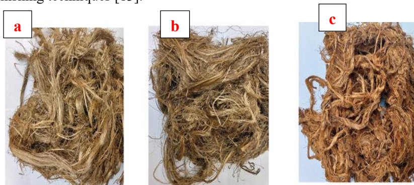
Fig. 3. Extracted banana fibers (a) Water retting, (b) Boiling in water (c) Caustic soda aqueous solution [14]
