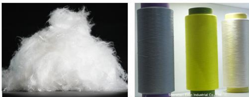
Fig. 3: PLA short fibers and filaments [8]
